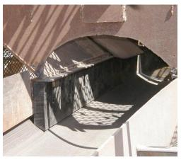
An operation in West Arkansas experienced extensive material spillage, dusting issues, and challenges keeping material centered on the belt. In an effort to solve these problems, the operation tried various sealing options in the interior transfer area, including conveyor belts, but they only lasted 6-8 weeks. The 6 ½" minus material from the Primary was running at 400 TPH.
