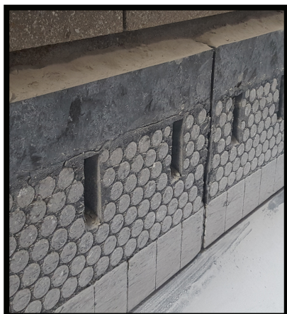
Rubber-Ceramic Canoe Liners
