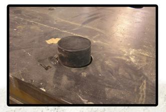
Rubber plugs are provided for each counterbored hole to protect the hardware. Use water on the plugs to make them slip in with ease.
